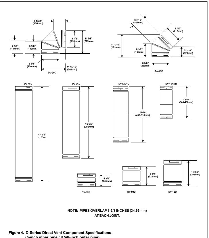
(5-inch inner pipe / 8 5/8-inch outer pipe)
